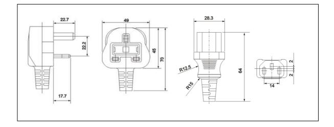
End 1: UK Moulded Plug Black Fuse: 5A Fuse Lead: 2,00mts HO5VV-F 3x0,75 black End 2: IEC Cold Connector (C13) black
